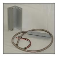
N/O, N/C Loop SPDT (Form C) Switch concealed with polished aluminum die-cast housing. Magnet mounted on adjustable L angle bracket. 24" Stainless armored cable.
